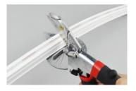
Use professional scissors to cut vertically at the cutting mark
