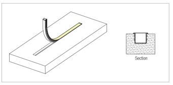
3.Align the light to the groove, press the glowing surface of the light, and fully embed the light into the groove.
